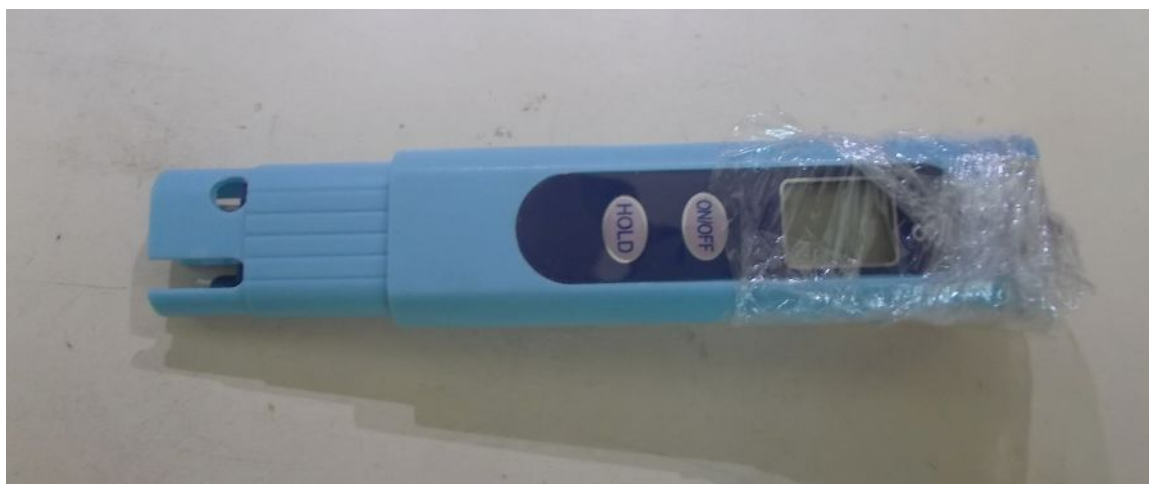
A very cheap EC meter, converted to use one CR2032 (a lithium coin cell will not leak as easily as alkaline LR44 cells.) Good enough for non-scientific work.
